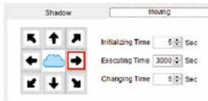
Select the moving direction of the cloud, initialization time, running time and the time interval of cloud moving
