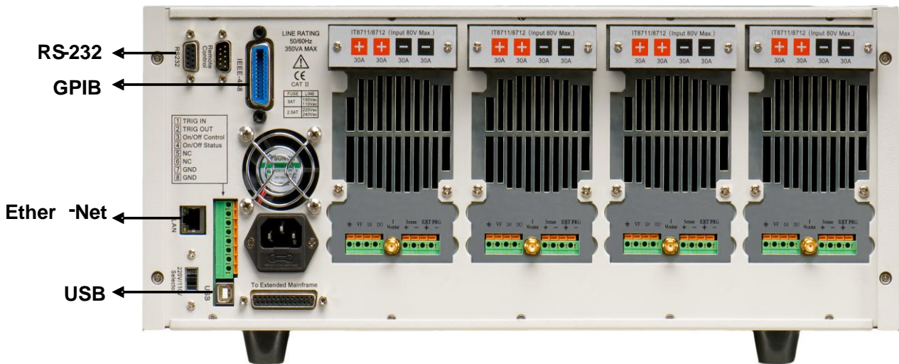
Figure 7-1IT8700 rear panel communication interface (take example of IT8702)
