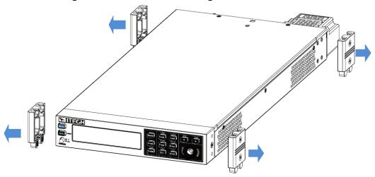
After the side footings are removed from the instrument, the user can see the rack mounting holes on both sides of the instrument.
