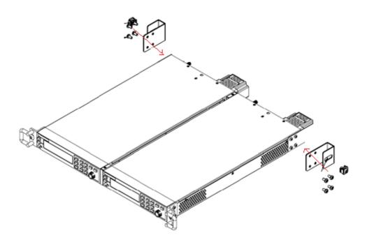
3. Based on the steps shown below, combine two sets of instruments mounted with left and right rack accessories. Use screws to fix the front and rear ends of the two sets of instruments from up to down.
