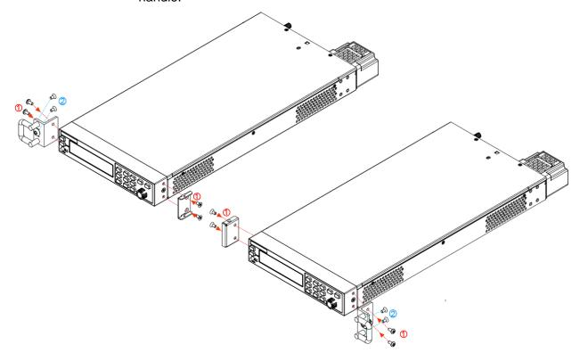
3. As shown below, combine two sets of instruments mounted with left and right racks. Use screws to fix the two sets of instruments from up to down.
