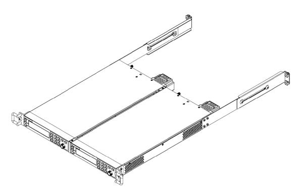
5. The user may install the rack-mounted instrument on a standard cabinet. The size for rack-mounted instrument is as shown below. (Unit: mm)
