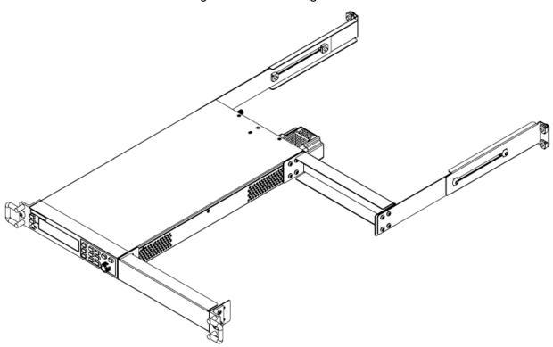
4. The user may install the rack-mounted instrument on a standard cabinet. The size for rack-mounted instrument is as shown below. (Unit: mm)
