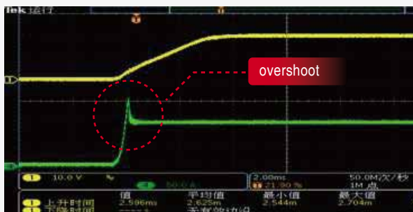
Diode load Conventional power test
